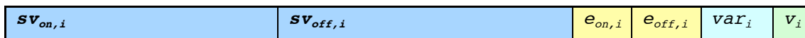
Figure 3.9: Feature vector fv_i created from the i :th segment of the input signal.
